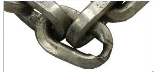
The chain link is heavily worn.
