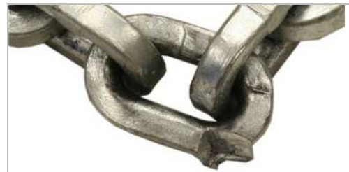
The chain link is mechanically damaged.
